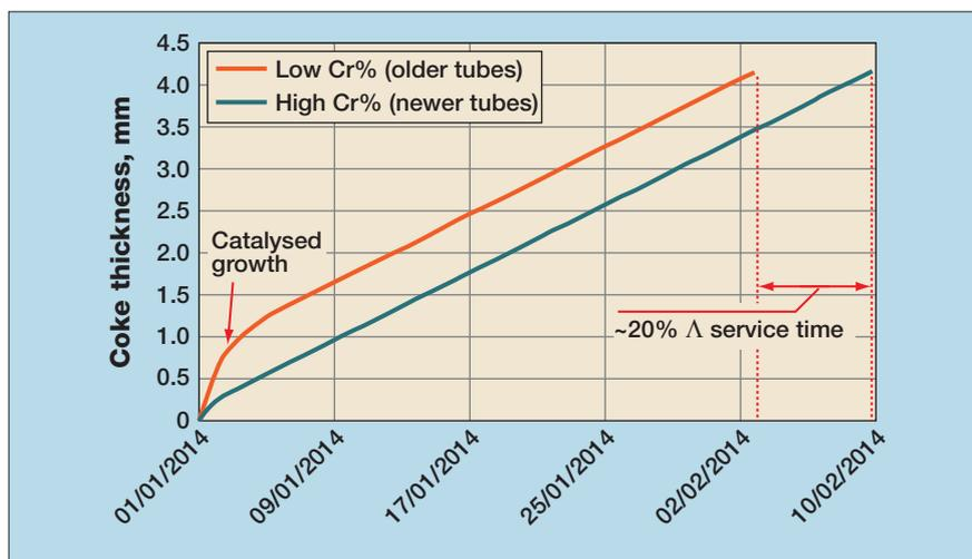
Figure 2 New vs old tube coke growth profiles
