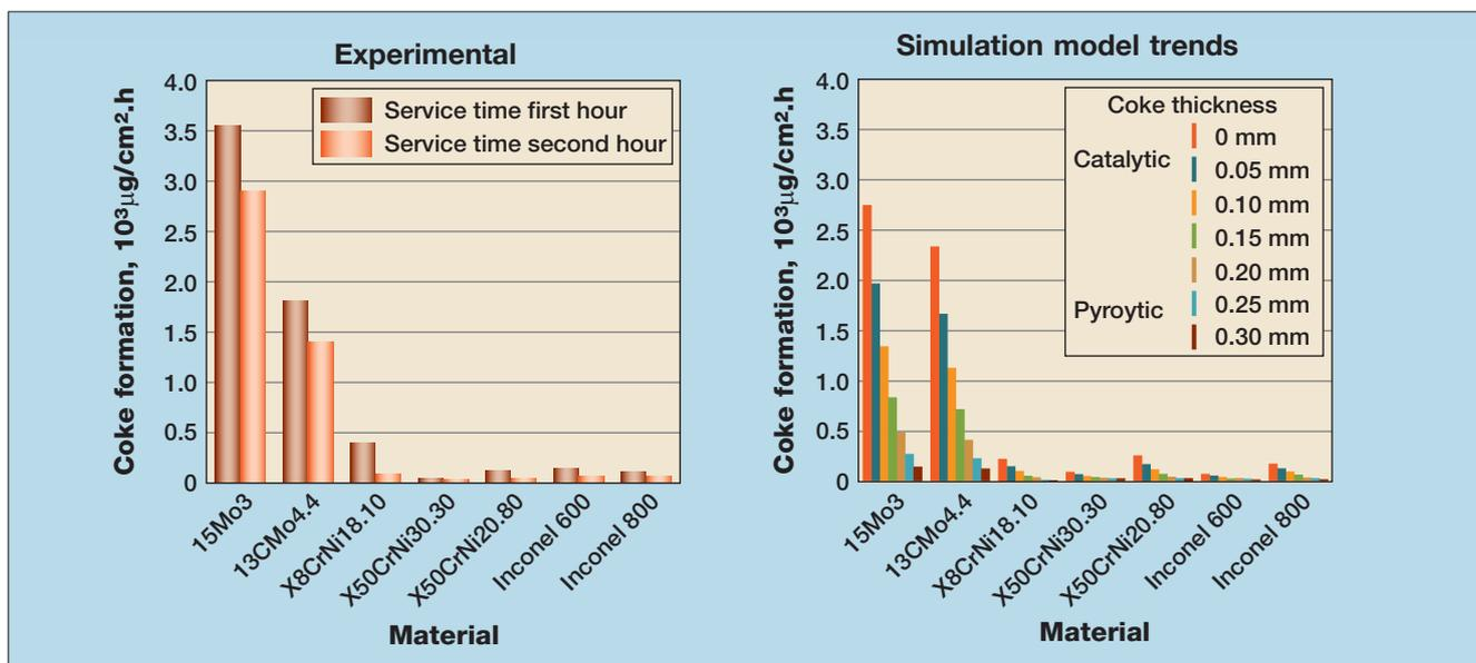
Figure 1 Pyrolytic versus catalytic coke growth model comparisons
