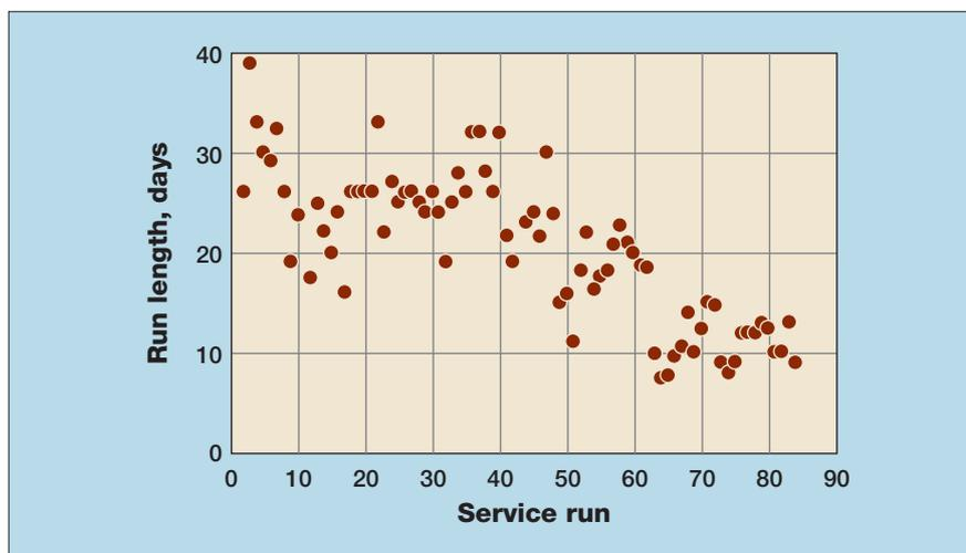
Figure 3 Run length for ethane feed unit in terms of service run (with outliers removed)
