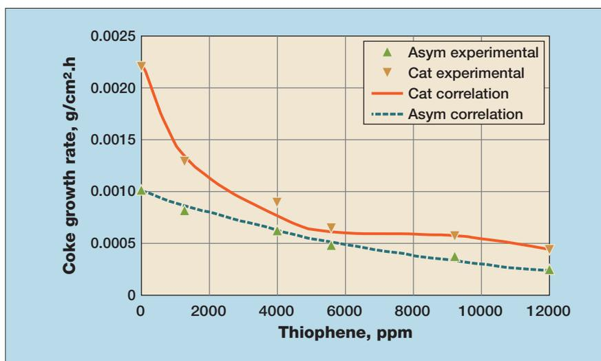
Figure 4 Coke formation rate as a function of thiophene inhibitor for two types of asymptotic and catalytic coke formation (experimental data<sup>11</sup> and correlation given in Eq.2)
